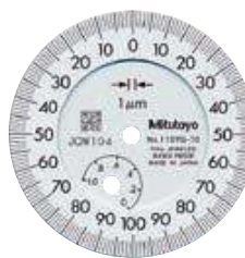
Graduation: 0.001mm, Measuring range: 1mm 1109S-10 Shockproof Jeweled bearing
